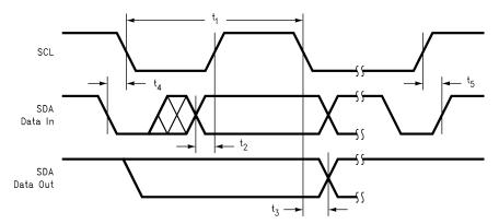
Figure 4. Serial Bus Communication
