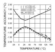
Figure 3. Accuracy vs Temperature with  $+V_s = 3.3V$
