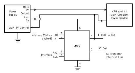
Figure 19. ACPI Compatible Terminal Alarm Shutdown
