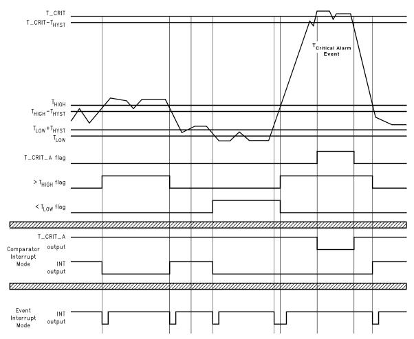
**Note:** Event Interrupt mode is drawn as if the user is reading the part. If the user doesn't read, the outputs would go low and stay that way until the LM92 is read. Comparator Interrupt Mode is drawn as if the user never reads the part. If the user does read, the outputs will go high once read instruction is executed and, if the fault condition still exists, go low at the end of the next conversion.
